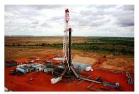
enough to support commercial production. The cost of producing shale gas in Australia is likely to be higher than for other resources, because of the need to acquire technology to undertake the complicated process of smashing the rocks open with sand, chemicals and water in a process known as hydraulic fracturing, or fracking.
